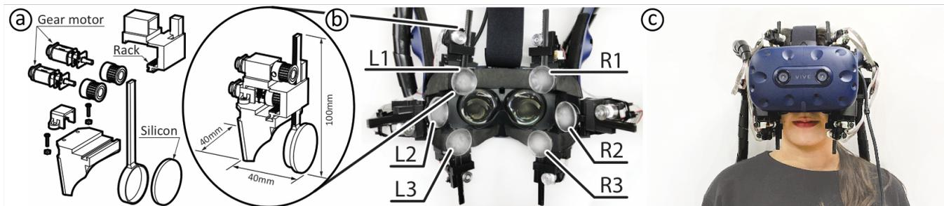
Figure 3. The Masque prototype actuates three pairs of skin stretch modules. The (a) exploded view and (b) the hardware implementation of the skin stretch module. (c) A user wears the Masque prototype.
