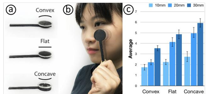
**Figure 2.** (a) The shear factors we explored, including convex, flat, and concave shapes. (b) The participant generates skin stretches by the factors. (c) User preferences regarding the shear factors. Error bars show a standard error in all figures.
