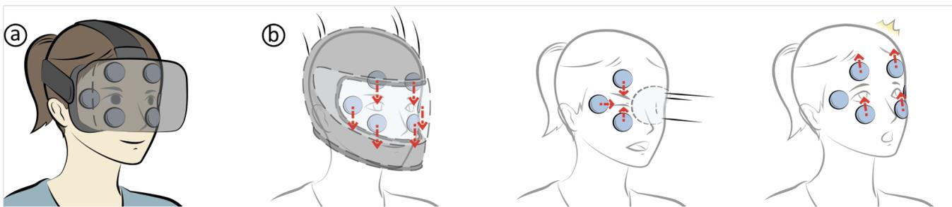
**Figure 1.** Masque is a prototype HMD integrating with six skin stretch modules. (a) Six shear factors are placed on the facial interface and can generate 2-degree-of-freedom lateral skin stretches, (b) which enables various skin stretch feedback or directional cues in virtual reality.
