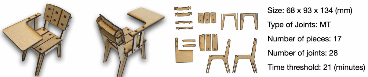
Figure 16: Details of each chair used as our representative laser-cut architecture examples. In a top-down order, the chairs were named based on the types of joint: Finger, Slot, MT, FingerMT and SlotMT in this paper.
