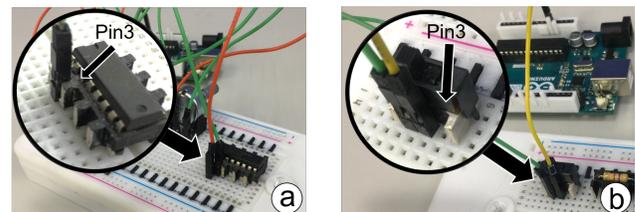
Figure 14: Hard to find pin<sub>3</sub> when (a) there is a wire header inside pin<sub>2</sub> slot or (b) the neighbouring slots were taken.
