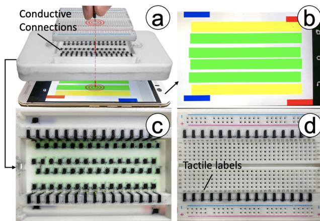
**Figure 7: (a) AccessibleCircuits audio-haptic interface displayed on a commodity smartphone overlaid with the 3D printed adaptation (b) Smartphone interface. (c) Top-view of extension case. Each black squares is printed in conductive filament. (d) Encased breadboard and tactile labels.**
