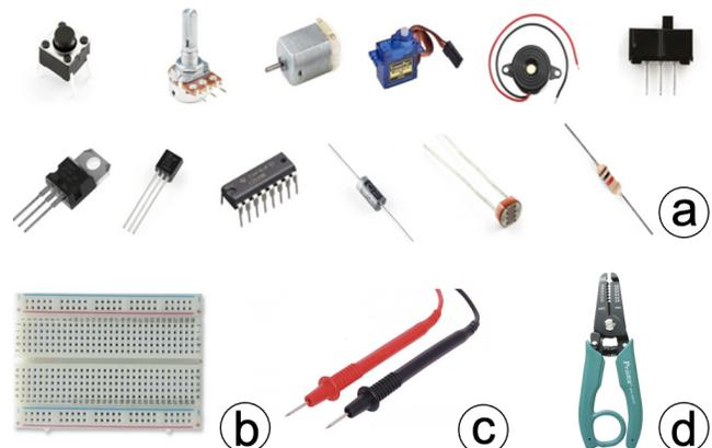
**Figure 2:** (a) Components include a button, potentiometer, motor, servo, buzzer, slide switch, transistor, temperature sensor, 16-pins IC, diode, photocell, resistor, (b) half-size breadboard, (c) probes, (d) and a wire stripper.
