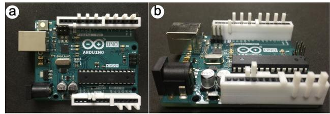
**Figure 8: Adaptations with tactile labels for Arduino UNO.**
