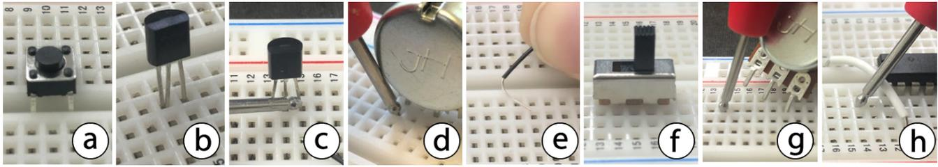
**Figure 6:** (a) P4 inserted the button cross the groove of the breadboard and confidently thought it was completed. (b) P1 inserted two pins of temperature sensor into the same hole. (c) The pins of temperature sensor are too thin to be felt by probe. (d) The pins of potentiometer are occluded by the body. (e) The end of wires is easily bent. (f) The pins of the slide switch are hidden. (g) Component bumped off the breadboard. (h) Wires can hinder the movement of probe.
